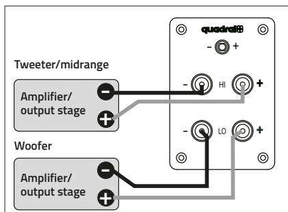
During Bi-wiring / Bi-amping operation of the **AURUM** loudspeaker, both screw terminals for the woofer (LO) are below and for the midrange speakers and tweeters (HI) are above on the connection plate.
